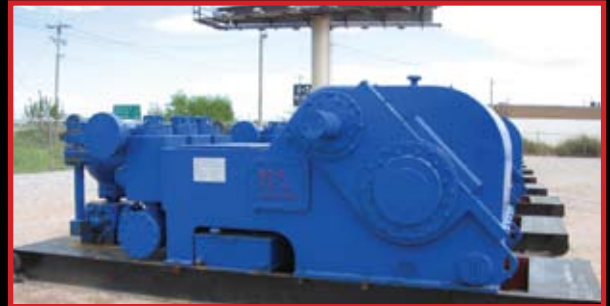
(14) MZ9 TRIPLEX PUMPS
