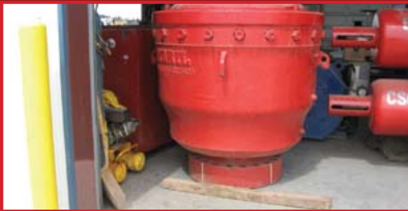
HYDRIL ANNULAR 13 5/8" 5K WITH 13 5/8" 10K FLANGE
